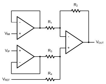
Figure 6. Instrument Amplifier
