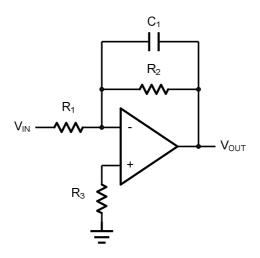
Figure 5. Low Pass Active Filter
