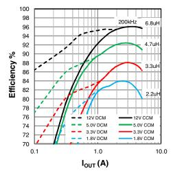
Figure 22: XR76205-Q Efficiency,  $V_{IN} = 24V$
