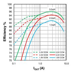
Figure 19: XR76208-Q Efficiency, V<sub>IN</sub> = 12V
