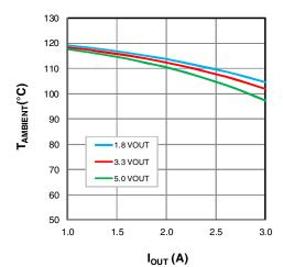
Figure 29: XR76203-Q, V<sub>IN</sub> = 12V
