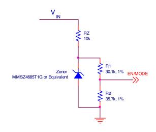
Figure 31: Selecting Forced CCM by Deriving EN/MODE from VIN
