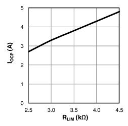
Figure 9: XR76203-Q I<sub>OCP</sub> versus R<sub>LIM</sub>
