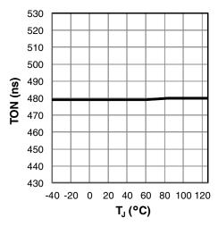
Figure 12:  $T_{ON}$  versus Temperature,  $R_{ON}$  = 35.7k $\Omega$
