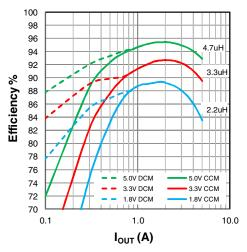
Figure 21: XR76205-Q Efficiency, V<sub>IN</sub> = 12V
