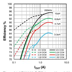
Figure 24: XR76203-Q Efficiency, V<sub>IN</sub> = 24V
