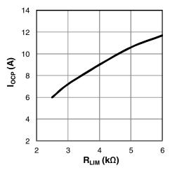
Figure 7: XR76208-Q  $I_{OCP}$  versus  $R_{LIM}$
