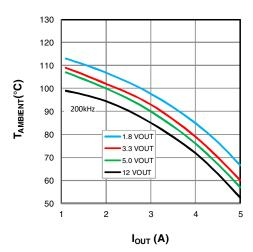
Figure 28: XR76205-Q, V<sub>IN</sub> = 24V
