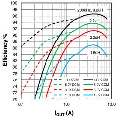
Figure 20: XR76208-Q Efficiency, V<sub>IN</sub> = 24V
