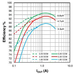
Figure 23: XR76203-Q Efficiency, V<sub>IN</sub> = 12V
