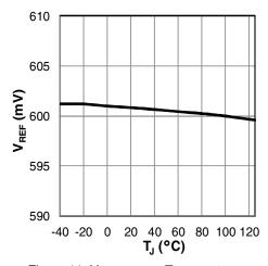
Figure 11: V<sub>REF</sub> versus Temperature
