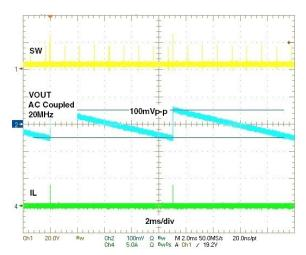
Figure 14: Steady State, DCM, I<sub>OUT</sub>=0A
