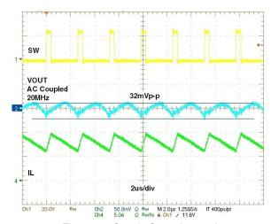
Figure 13: Steady State, I<sub>OUT</sub>=8A
