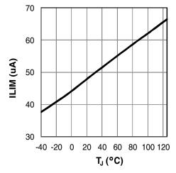
Figure 10: I<sub>LIM</sub> versus Temperature
