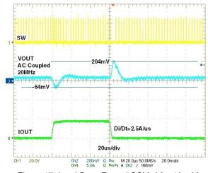
Figure 17: Load Step, Forced CCM, 0A - 4A - 0A
