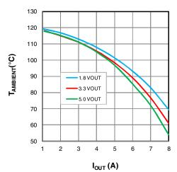
Figure 25: XR76208-Q, V<sub>IN</sub> = 12V
