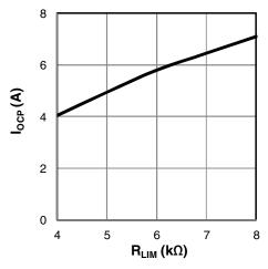
Figure 8: XR76205-Q  $I_{OCP}$  versus  $R_{LIM}$
