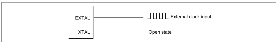
Figure 4.4 Example of External Clock Connection
