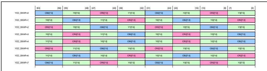
Figure 35.6 YCbCr422 Data Arrangement with Swapping Enabled
