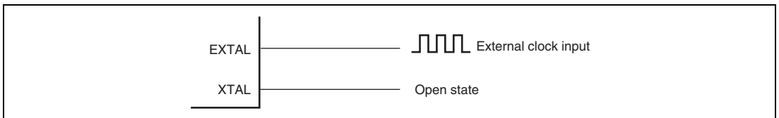
Figure 4.4 Example of External Clock Connection
