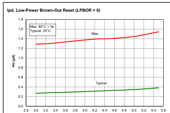
FIGURE 32-42: I_{PD} , LP Brown-Out Reset ( LPBOR = 0 ), PIC16F1788/9 Only.
