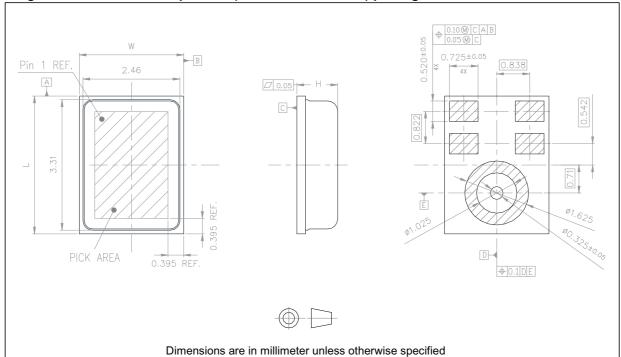
Dimensions are in millimeter unless otherwise specified General Tolerance is +/-0.15mm unless otherwise specified
