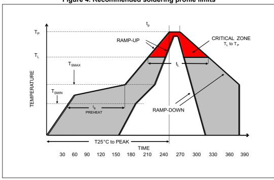
Figure 4. Recommended soldering profile limits
