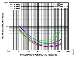
Figure 7. Gyroscope Allan Deviation,  $T_C = 25^{\circ}$ C, ADIS16505-1, Plot Taken After 10 Hours of Settling Time
