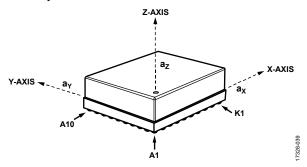
Figure 50. Accelerometer Axis and Polarity Assignments
