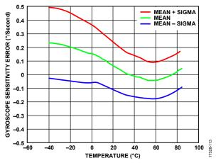
Figure 13. Gyroscope Sensitivity Error vs. Temperature, ADIS16505-1,
