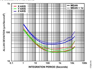
Figure 23. Accelerometer Allan Deviation,  $T_C = 25^{\circ}C$
