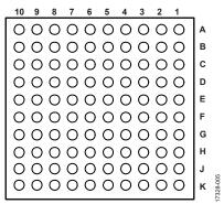
Figure 5. Pin Assignments, Bottom View
