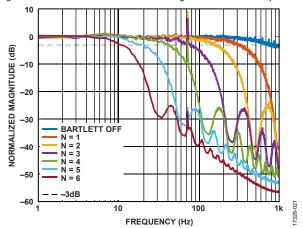
Figure 28. Accelerometer Normalized Noise Density
