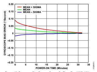
Figure 17. Gyroscope Bias Error vs. Power-On Time,  $T_C = 25$ °C, All Axes
