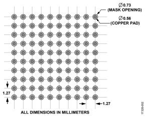
Figure 62. Recommend PCB Pattern, Solder Mask Defined Pads
