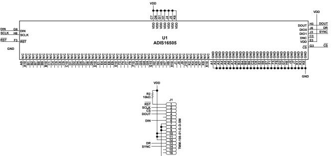
Figure 65. ADIS16505 Breakout Board Schematic
