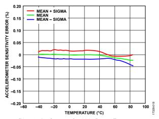
Figure 25. Accelerometer Sensitivity Error vs. Temperature, Cold to Hot, All Axes
