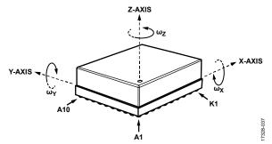
Figure 48. Gyroscope Axis and Polarity Assignments
