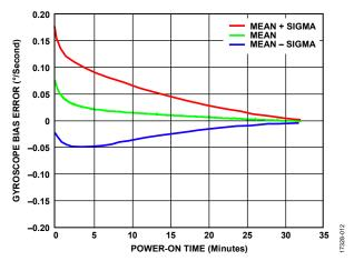
Figure 18. Gyroscope Bias Error vs. Power-On Time,  $T_C = 85$ °C, All Axes
