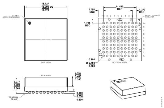
Figure 66. 100-Ball Ball Grid Array Module [BGA] (ML-100-1) Dimensions shown in millimeters
