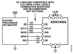
Figure 34. Electrical Connection Diagram
