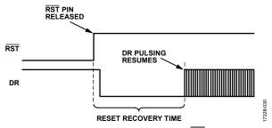
Figure 38. Data Ready Response During Reset ( $\overline{RST} = 0$ ) Recovery
