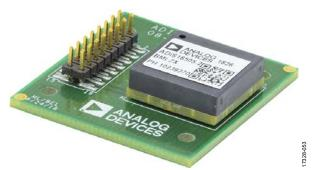
Figure 63. ADIS16505-2 Breakout Board
