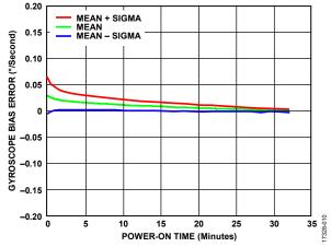
Figure 16. Gyroscope Bias Error vs. Power-On Time,  $T_C = -40$ °C, All Axes
