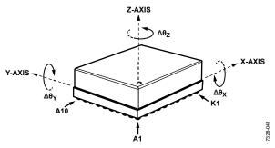
Figure 52. Delta Angle Axis and Polarity Assignments
