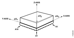
Figure 54. Delta Velocity Axis and Polarity Assignments
