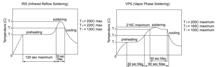
Note: 1.Temperature profiles show the temperature of PC board surface.
