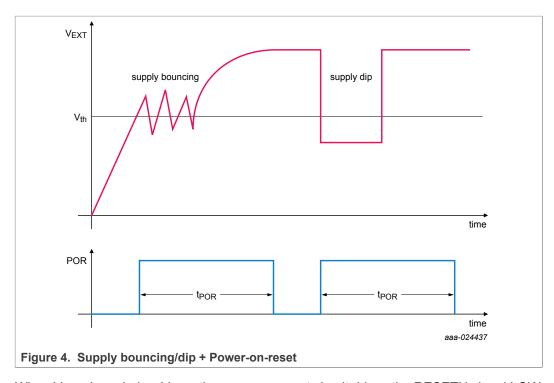
When  $V_{EXT}$  drops below  $V_{POR}$ , the power-on reset circuit drives the RESETN signal LOW weakly to generate a clean reset signal to reset the PMU. The PMU prolongs the reset for  $t_{POR}$  to reset the rest of the chip. When not active, the power-on reset circuit is driving the RESETN signal weakly HIGH (see <u>Figure 5</u>).
