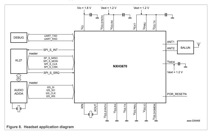
Ultra-low power 2.4 GHz Bluetooth Low Energy transceiver for audio streaming
