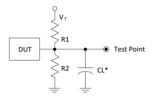
\*CL Includes Test Fixture and Probe Capacitance
