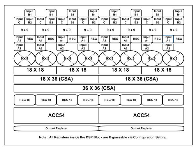
Figure 2.16. Certus-NX DSP Functional Block Diagram
