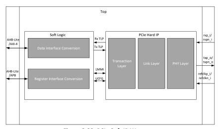
Figure 2.29. PCIe Soft IP Wrapper
