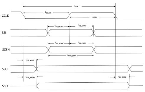
Figure 3.19. Slave SPI Configuration Timing
