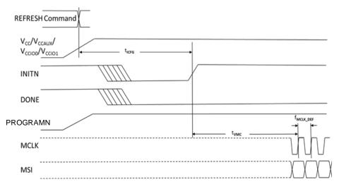
Figure 3.14. Master SPI POR/REFRESH Timing
