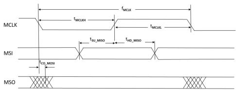
Figure 3.18. Master SPI Configuration Timing
