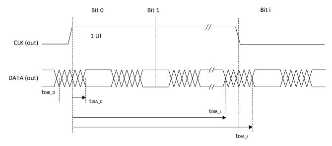
Figure 3.13. Transmitter DDRX71\_TX Waveforms
