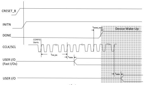
Figure 3.22. Slave SPI/I<sup>2</sup>C/I3C Wake-Up Timing
