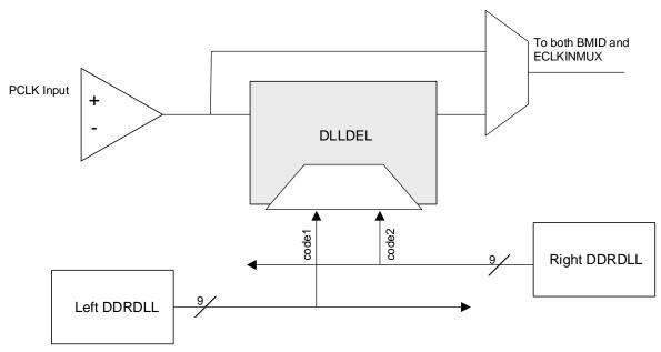
Figure 2.11. DLLDEL Functional Diagram
