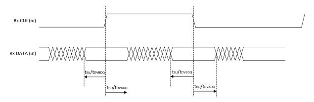
Figure 3.7. Receiver RX.CLK.Centered Waveforms
