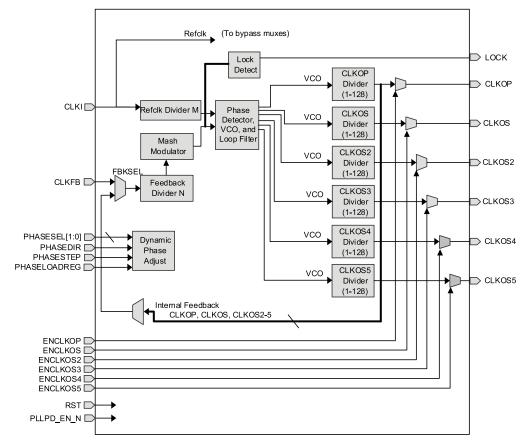
Figure 2.6. General Purpose PLL Diagram
