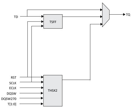
Figure 2.24. Tristate Register Block on Bottom Side
