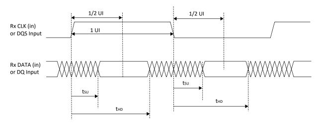
Figure 3.8. Receiver RX.CLK.Aligned and DDR Memory Input Waveforms
