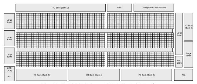
Figure 2.2. Simplified Block Diagram, LFD2NX-17 Device (Top Level)
