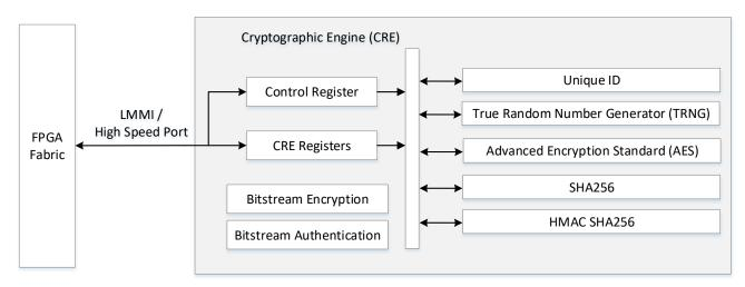
Figure 2.30. Cryptographic Engine Block Diagram
