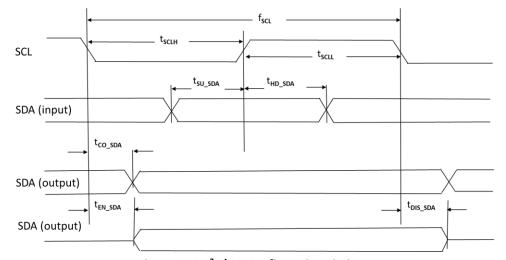
Figure 3.20. I<sup>2</sup>C/I3C Configuration Timing
