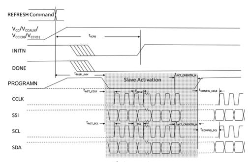
Figure 3.15. Slave SPI/I<sup>2</sup>C/I3C POR/REFRESH Timing
