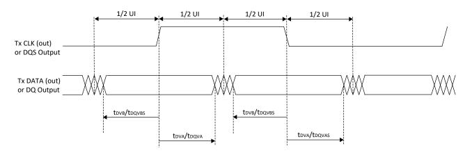
Figure 3.9. Transmit TX.CLK.Centered and DDR Memory Output Waveforms
