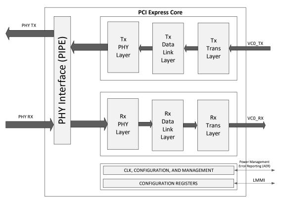
Figure 2.28. PCIe Core
