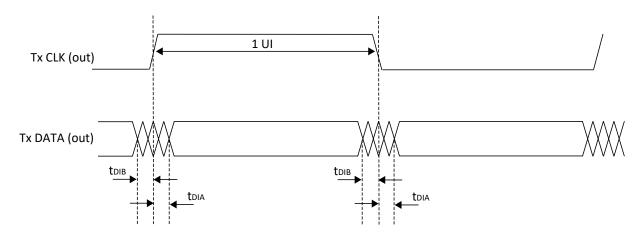
Figure 3.10. Transmit TX.CLK.Aligned Waveforms
