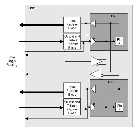
Figure 2.18. Wide Range Programmable I/O Cells
