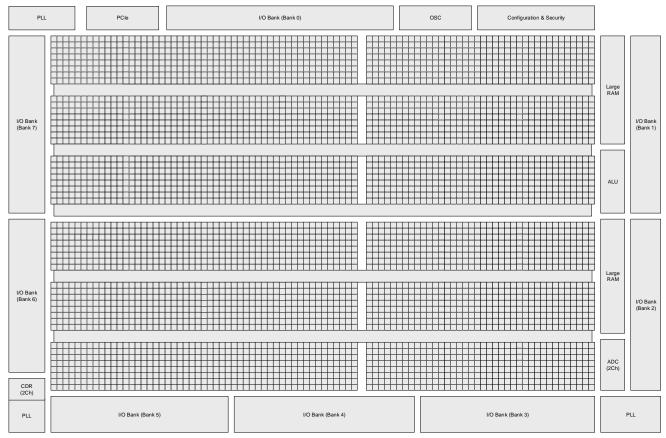
Figure 2.1. Simplified Block Diagram, LFD2NX-40 Device (Top Level)
