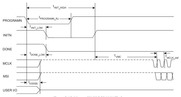
Figure 3.16. Master SPI PROGRAMN Timing
