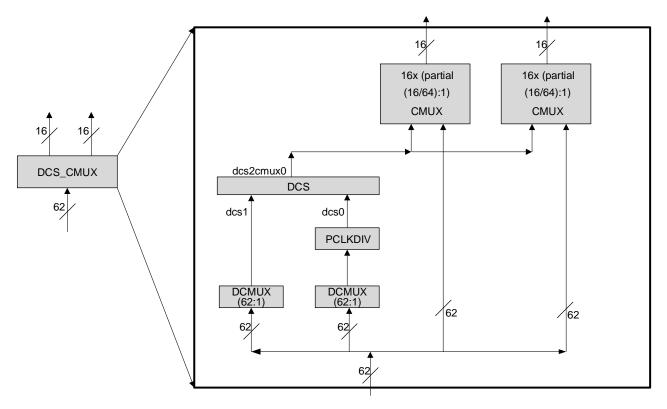
Figure 2.9. DCS\_CMUX Diagram
