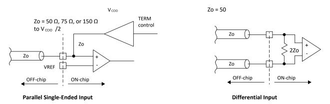
Figure 3.1. On-Chip Termination
