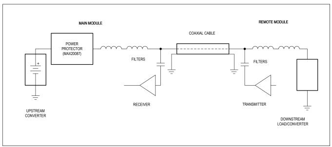
Figure 6. Example of System Architecture Diagram
