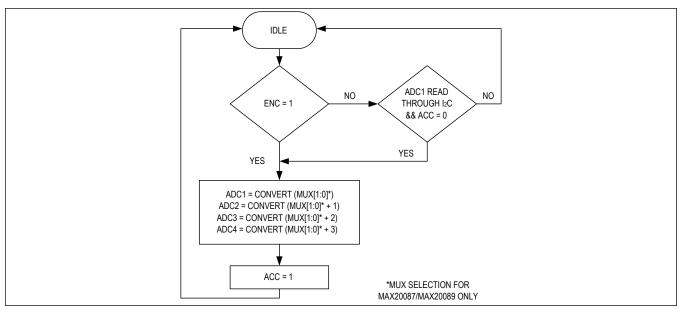
Figure 5. ADC Flow Diagram
