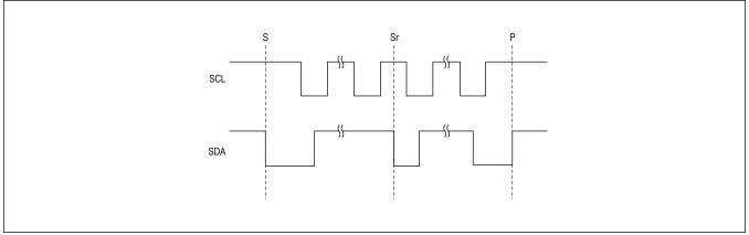
Figure 2. START, STOP, and Repeated START Conditions
