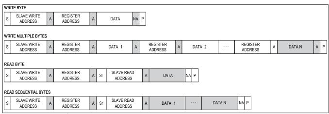
Figure 4. Data Format of I<sup>2</sup>C Interface
