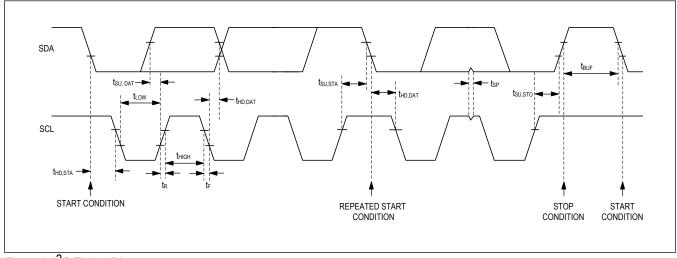
Figure 1. I<sup>2</sup>C Timing Diagram
