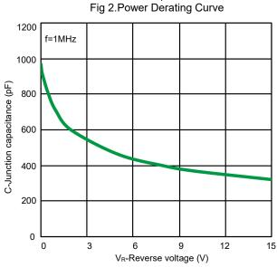
Fig 4. Capacitance vs. Reveres voltage
