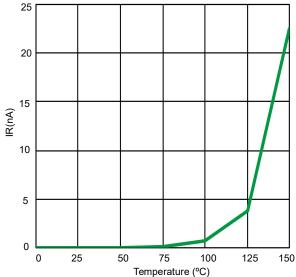
Fig 6.Typical Leakage Current vs. Temperature
