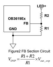
R2 — The resistor connected between the FB pin and the Output, the value suggested is 200Kohms~330Kohms
