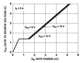
Figure 7. Gate Charge Characteristics
