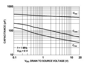
Figure 8.Capacitance vs Drain to Source Voltage
