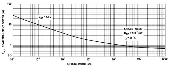
Figure 11. Single Pulse Maximum Power Dissipation
