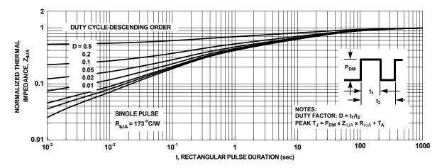
Figure 12. Junction to Ambient Transient Thermal Response Curve
