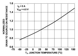
Figure 3. Normalized On-Resistance vs Junction Temperature
