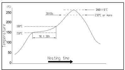
Temperature profile for reflow soldering
