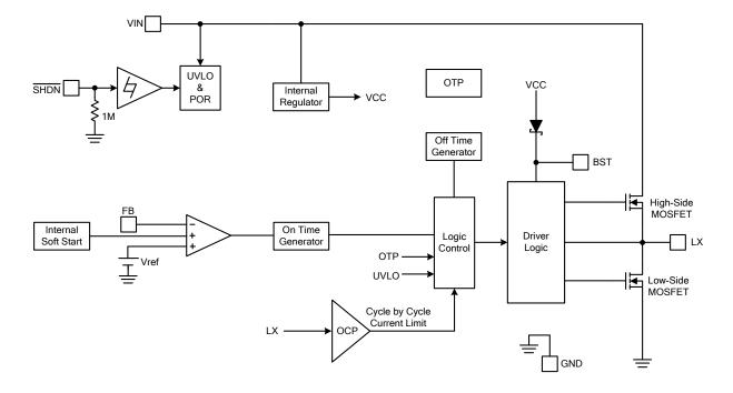
Figure 3. Block Diagram of EA9206
