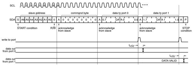
Figure 6. Write to Output Port Registers
