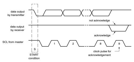
Figure 17. Acknowledgement of the I<sup>2</sup>C Bus
