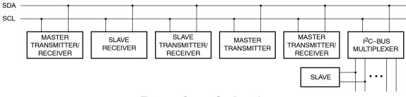
Figure 16. System Configuration
