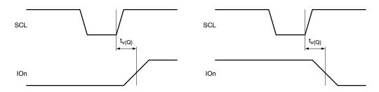
Figure 20. t<sub>V(Q)</sub> Timing
