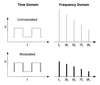
Figure 42. Spread Spectrum Comparison
