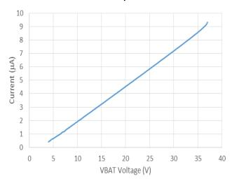
Figure 5. Shutdown V<sub>BAT</sub> Quiescent Current vs. V<sub>BAT</sub> Voltage
