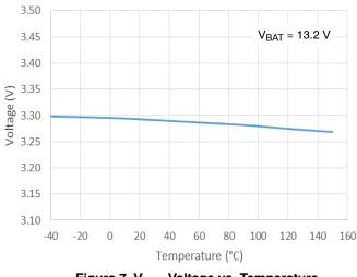
Figure 7. V<sub>DRV</sub> Voltage vs. Temperature
