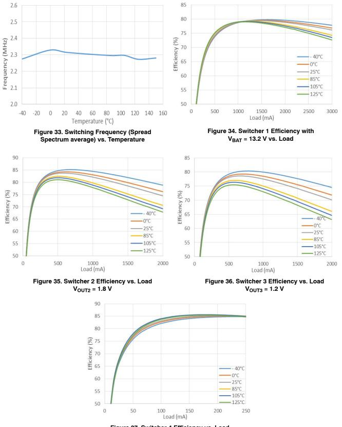
Figure 37. Switcher 4 Efficiency vs. Load
