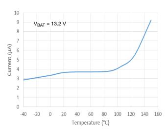
Figure 3. Shutdown V<sub>BAT</sub> Quiescent Current vs. Temperature
