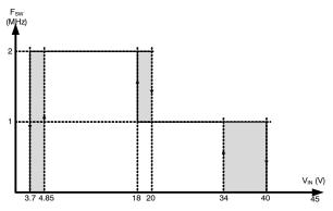
Figure 53. High Voltage Frequency Foldback
