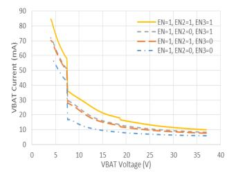
Figure 6. Operating V<sub>BAT</sub> Quiescent Current vs. V<sub>BAT</sub> Voltage
