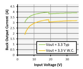
Figure 51. Switcher 1 Dc Output Current vs. VIN with a 4.7  $\mu H$  Inductor
