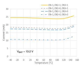
Figure 4. Operating V<sub>BAT</sub> Quiescent Current vs. Temperature
