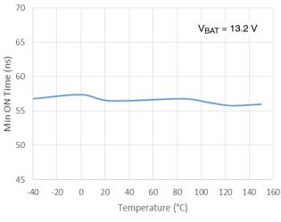
Figure 8. Switcher 1 Min ON Time vs. Temperature
