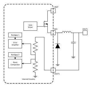
Figure 48. Switcher 1 Block Diagram
