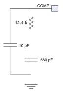
Figure 49. Recommended Compensation for Switcher 1
