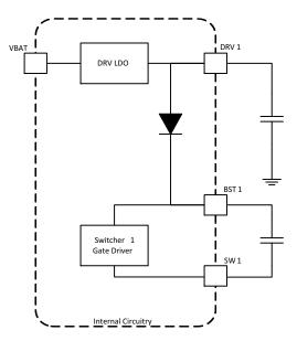
Figure 50. Switcher 1 Drive and Bootstrap Circuitry
