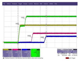
Figure 41. Soft Start Timing with Automatic Sequencing
