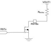
Figure 45. Reset Delay Circuit
