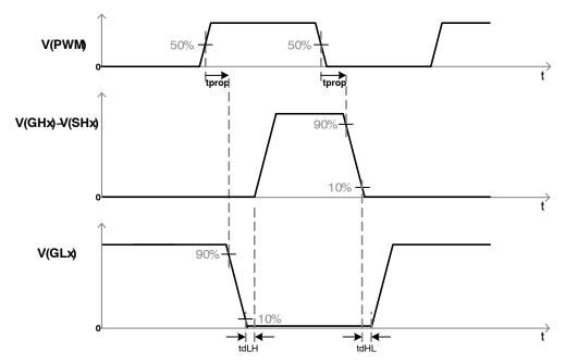
**Figure 2. Cross Conduction Protection Timing**
