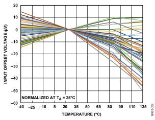
Figure 18. Input Offset Voltage vs. Temperature for 50 Devices
