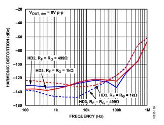
Figure 72. Harmonic Distortion vs. Frequency for Various R<sub>F</sub> and R<sub>G</sub> Values
