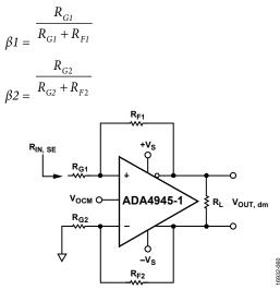
Figure 104. ADA4945-1 with Unbalanced (Single-Ended) Input
