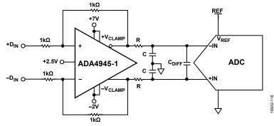
Figure 116. ADA4945-1 Driving Precision ADC
