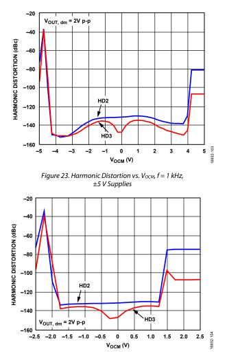
Figure 24. Harmonic Distortion vs.  $V_{OCM}$ , f = 1 kHz, ±2.5 V Supplies
