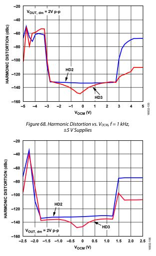
Figure 69. Harmonic Distortion vs.  $V_{OCM}$ , f = 1 kHz,  $\pm 2.5$  V Supplies
