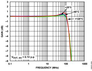
Figure 6. Small Signal Frequency Response for Various Temperatures
