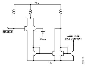
Figure 110. DISABLE Pin Circuit
