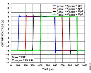
Figure 44. Large Signal Transient Response for Various Capacitive Loads,  $V_S = 10 V$
