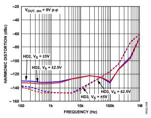
Figure 66. Harmonic Distortion vs. Frequency for Various Supplies
