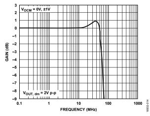
Figure 11. Large Signal Frequency Response at Various V<sub>OCM</sub> Levels
