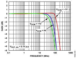
Figure 55. Small Signal Frequency Response at Various V<sub>OCM</sub> Levels
