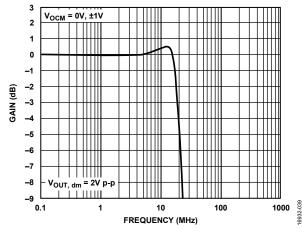
Figure 56. Large Signal Frequency Response at Various V<sub>OCM</sub> Levels
