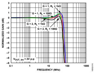
Figure 7. Large Signal Frequency Response for Various Gains and Loads
