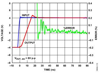
Figure 36. 0.1% Settling Time
