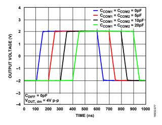
Figure 46. Large Signal Transient Response for Various Capacitive Loads,  $V_S = 3 V$
