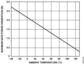
Figure 2. Maximum Safe Power Dissipation vs. Ambient Temperature
