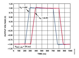
Figure 48. Vocm Large Signal Transient Response
