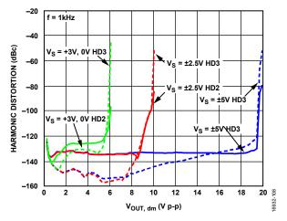
Figure 71. Harmonic Distortion vs.  $V_{OUT, dm}$  for Various Supplies, f = 1 kHz
