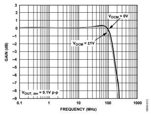
Figure 10. Small Signal Frequency Response at Various V<sub>OCM</sub> Levels
