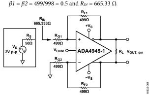
Figure 105. Single-Ended Input Impedance R<sub>IN</sub>
