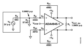
Figure 109. Terminated Single-Ended-to-Differential System with G = 1
