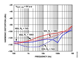
Figure 20. Harmonic Distortion vs. Frequency for Various Loads
