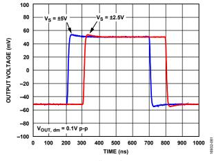
Figure 47. V<sub>OCM</sub> Small Signal Transient Response
