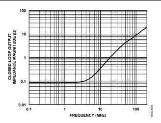
Figure 37. Closed-Loop Output Impedance Magnitude vs. Frequency, G = 1
