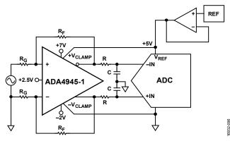
Figure 113. ADA4945-1 Output Voltage Clamp Usage
