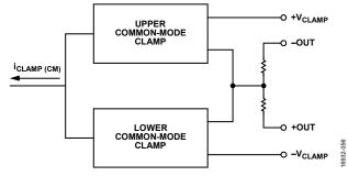
Figure 100. Common-Mode Clamp Block Diagram
