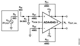
Figure 106. Adding Termination Resistor, R<sub>T</sub>
