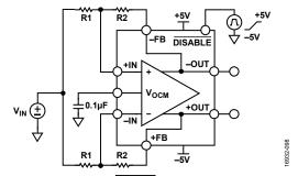
Figure 97. Test Circuit for DISABLE Pin Turn On Time Measurement
