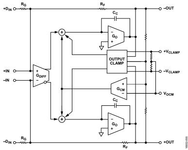
Figure 99. ADA4945-1 Architectural Block Diagram
