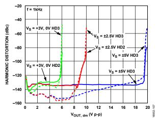
Figure 26. Harmonic Distortion vs.  $V_{OUT, dm}$  for Various Supplies, f = 1 kHz
