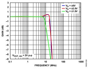
Figure 53. Large Signal Frequency Response for Various Supplies
