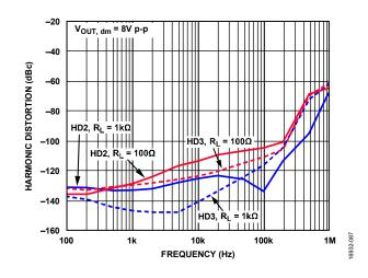
Figure 65. Harmonic Distortion vs. Frequency for Various Loads
