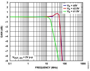
Figure 8. Large Signal Frequency Response for Various Supplies
