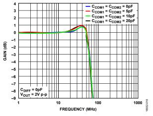
Figure 15. Large Signal Frequency Response for Various Capacitive Loads
