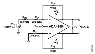
Figure 108. Thevenin Equivalent with Matched Gain Resistors
