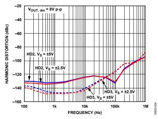
Figure 21. Harmonic Distortion vs. Frequency for Various Supplies
