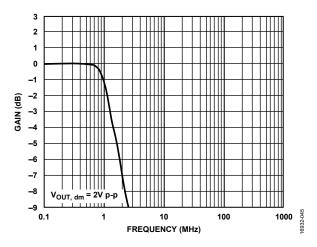
Figure 62. V<sub>OCM</sub> Large Signal Frequency
