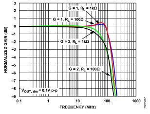
Figure 4. Small Signal Frequency Response for Various Gains and Loads
