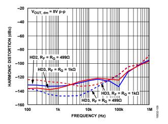
Figure 27. Harmonic Distortion vs. Frequency for Various R<sub>F</sub> and R<sub>G</sub> Values
