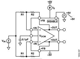
Figure 96. Test Circuit for DISABLE Pin Turn Off Time Measurement
