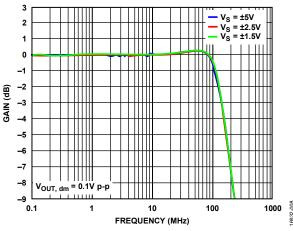
Figure 5. Small Signal Frequency Response for Various Supplies
