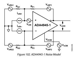
As with conventional op amps, the output noise voltage densities can be estimated by multiplying the input referred terms at +IN and –IN by the appropriate output factor, where:
