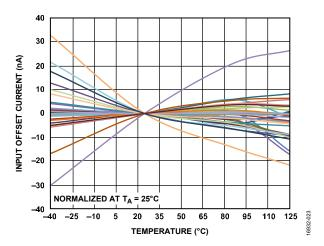
Figure 19. Input Offset Current vs. Temperature for 30 Devices
