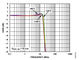
Figure 54. Large Signal Frequency Response for Various Temperatures
