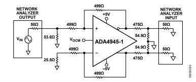
Figure 94. Equivalent Basic Test Circuit
