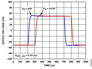
Figure 92. VOCM Small Signal Transient Response
