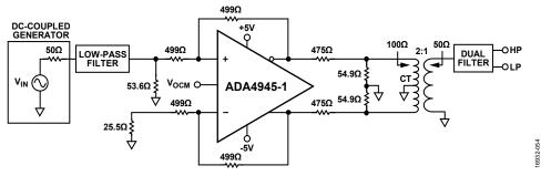
Figure 95. Test Circuit for Distortion Measurements
