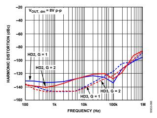
Figure 22. Harmonic Distortion vs. Frequency for Various Gains
