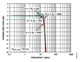
Figure 52. Large Signal Frequency Response for Various Gains and Loads
