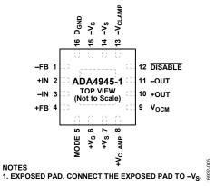
Figure 3. Pin Configuration
