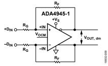
Figure 103. ADA4945-1 Configured for Balanced (Differential) Inputs
