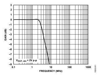
Figure 17. VOCM Large Signal Frequency Response
