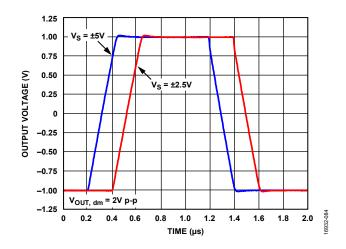
Figure 93. Vocm Large Signal Transient Response
