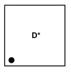
D= Device code \* = Month code (A~Z) Marking (Top view)
