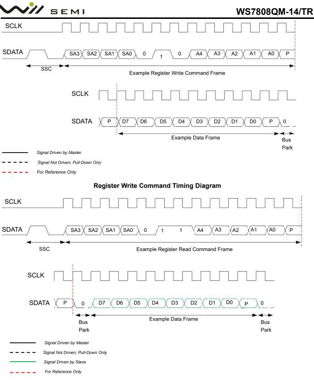
Register Read Command Timing Diagram
