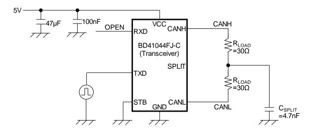
Figure 12. Evaluation Circuit Diagram
