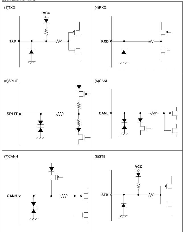
Figure 13. I/O Equivalent Circuits
