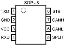
Figure 2. Pin Configuration(TOP VIEW)
