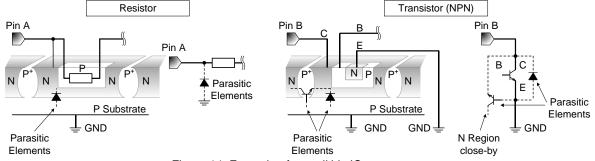
Figure 14. Example of monolithic IC structure
