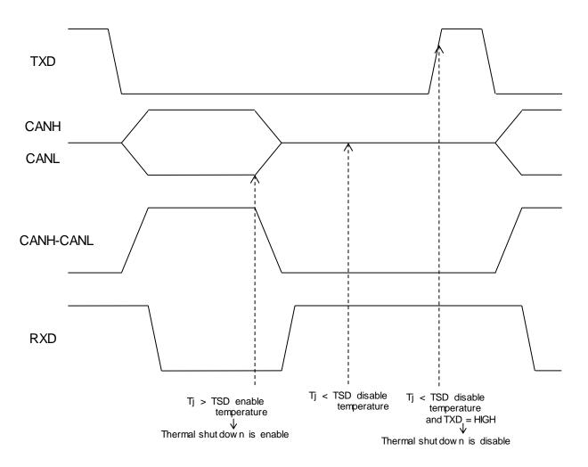
Figure 9. Thermal Shutdown Operating
