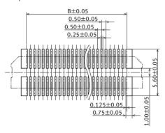
■ Recommended metal mask pattern Metal mask thickness: When 150 µm (Opening area ratio: 62%)
