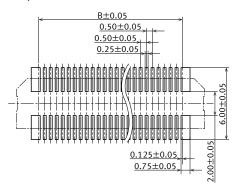
■ Recommended metal mask pattern Metal mask thickness: When 150 µm (Opening area ratio: 69%)
