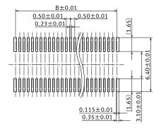
■ Recommended metal mask pattern Metal mask thickness: When 120 µm (Opening area ratio: 78%)
