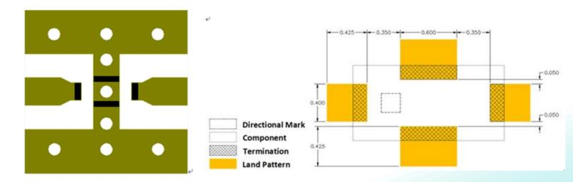
Line width should be designed to match  $50\Omega$  characteristic impedance, depending on PCB material and thickness.
