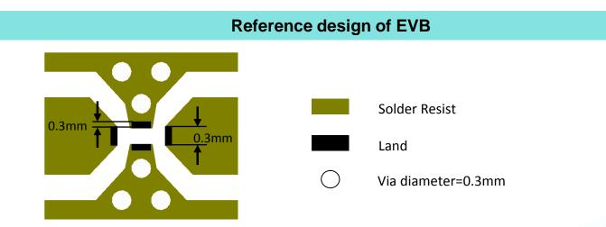
Line width should be designed to match  $50\Omega$  characteristic impedance, depending on PCB material and thickness.
