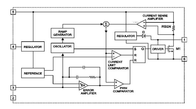
Figure 1 Function Block Diagram of TD1836
