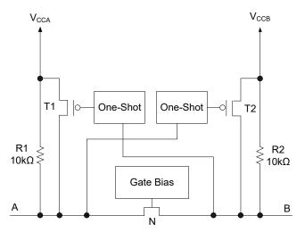
Figure 3. Architecture of a SGM4578 Cell
