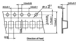
\*Dimension of the Cavity is measured at the bottom side. (in mm)
