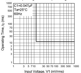
Operating Time vs. Input Voltage
