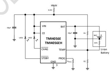
Figure 1. Basic Application Circuit
