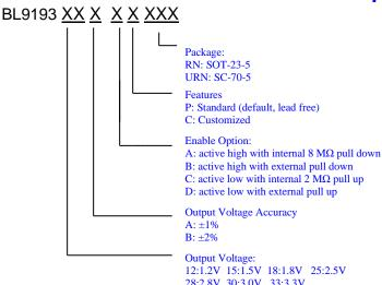
12:1.2V 15:1.5V 18:1.8V 25:2.5V 28:2.8V 30:3.0V 33:3.3V CT: custom fixed output (50mV step) AD: Adjustable
