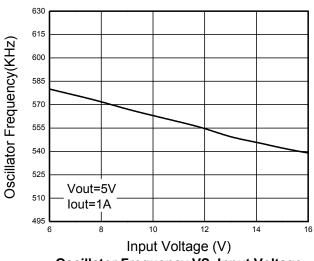
Oscillator Frequency VS. Input Voltage
