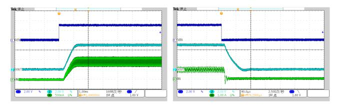
$V_{\text{IN}}$ =12V,  $V_{\text{O}}$ =5V, $V_{\text{EN}}$ =3.0V, $I_{\text{O}}$ =2A, EN On
