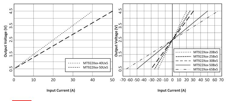
Figure.3 Output Voltage vs. Input Current
