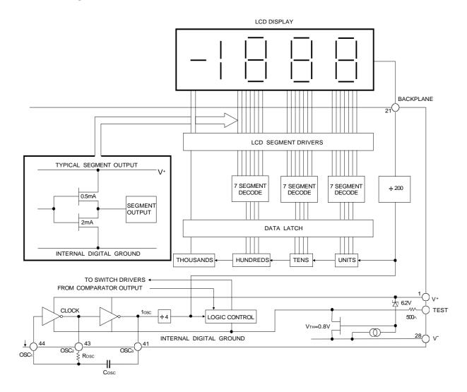
The internal digital ground is generated from a 6.2 volt Zener diode and a large p-channel follower. This supply is made stiff to adsorb the relatively large capacitive current when the back plane (BP) is switched. The BP frequency is the clock frequency divided by 800. The segments are driven at the same frequency and amplitude and are in phase with BP when OFF, but out of phase when ON. In all cases, negligible DC voltage exists across the segments.
