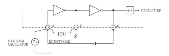
To achieve maximum rejection of 50/60 Hz pick up, the signal integrate cycle should be a multiple of 50/60 Hz. The following table describes the selection of oscillator frequencies for 50 or 60 Hz respectively.
