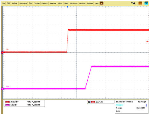
Startup by power-on
