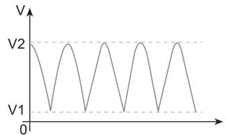
Here:  $V_1 \geq 0$ ,  $V_2 \leq U_R$ ,  $V_{rms} = (V_2 - V_1) \div \sqrt{2}$ ,  $I_{rms} = 2\pi f \times C \times (V_2 - V_1) \div \sqrt{2}$
