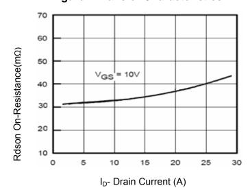
Figure 3 Rdson- Drain Current
