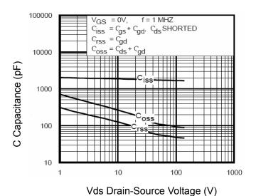
Figure 7 Capacitance vs Vds
