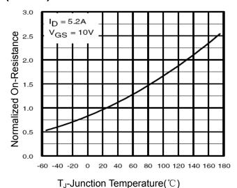
Figure 4 Rdson-JunctionTemperature
