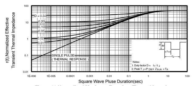
**Figure 11 Normalized Maximum Transient Thermal Impedance**
