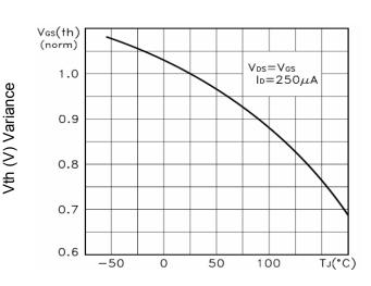
$\label{eq:TJ-Junction Temperature} T_{J}\mbox{-Junction Temperature}(^{\circ}\mbox{C}) $$ Figure 10 $V_{GS(th)}$ vs Junction Temperatur$
