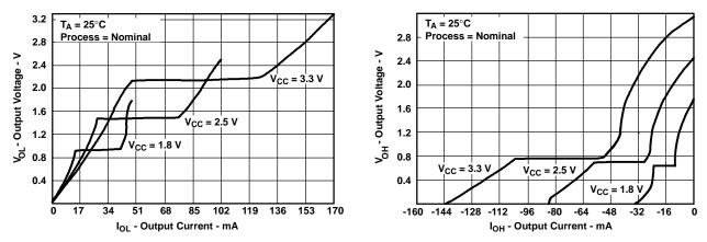
Figure 1. Output Voltage vs Output Current
