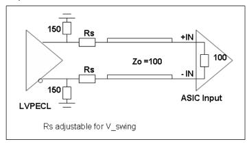
LVPECL V\_swing Adjustment using Rs
