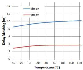
Figure 15. Delay Matching vs. Temperature
