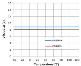
Figure 25. VBS UVLO vs. Temperature
