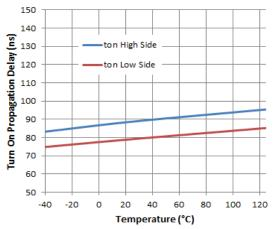
Figure 5. Turn-on Propagation Delay vs. Temperature
