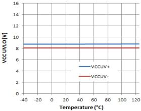
Figure 24. VCC UVLO vs. Temperature
