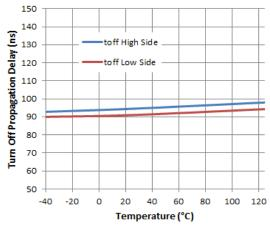
Figure 7. Turn-off Propagation Delay vs. Temperature
