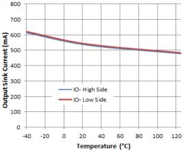
Figure 19. Output Sink Current vs. Temperature
