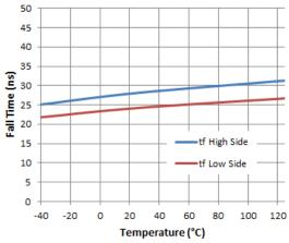
Figure 11. Fall Time vs. Temperature
