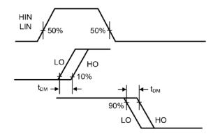
Figure 1. Input / Output Timing Diagram
