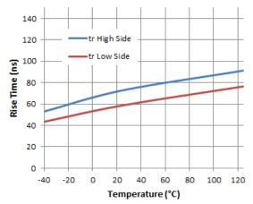
Figure 9. Rise Time vs. Temperature
