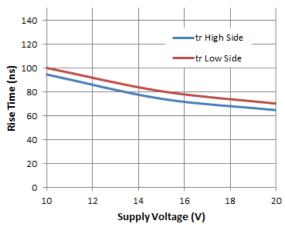
Figure 8. Rise Time vs. Supply Voltage
