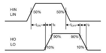
Figure 3. Switching Time Waveform Definitions
