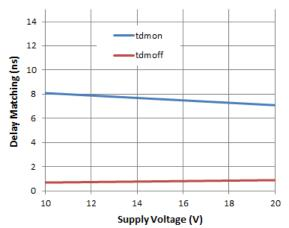
Figure 14. Delay Matching vs. Supply Voltage
