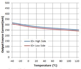
Figure 17. Output Source Current vs. Temperature
