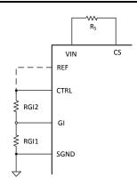
Figure 4. Setting LED Current
