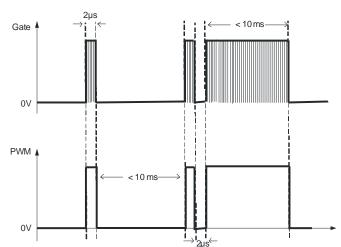
Figure 8. PWM Dimming Minimum and Maximum Pulse
