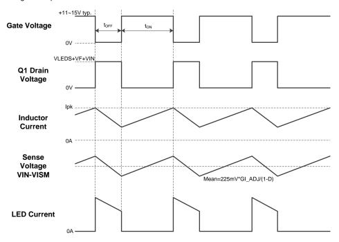
Figure 3. Operating Waveforms
