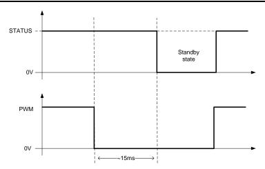
Figure 9. Stand-by State from PWM Signal
