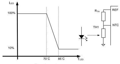
$\label{eq:Thermal network response:} R_{TH} = 1.8k\Omega \text{ and } TH1 = 10k\Omega \text{ (beta = 3900)}$
