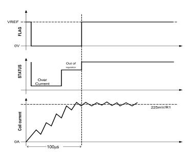
Figure 12. Diagnostic during Start-up
