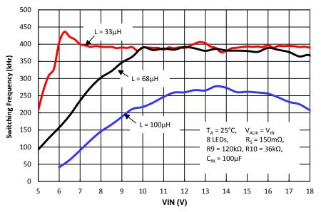
Figure 5. Frequency vs. VIN LED Driver with 350mA LED Current and Various Inductor Values
