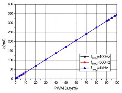
Figure 7. LED Current Linearity and Accuracy with PWM Dimming
