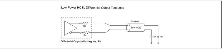
Figure 1. Low Power HCSL Test Circuit
