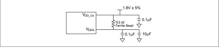
Figure 4. Power Supply Filter
