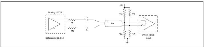
Figure 3. Differential Output driving LVDS
