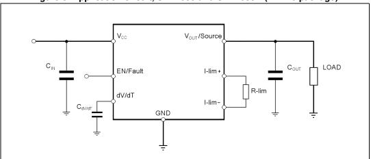
Figure 3. Application circuit, STEF033 and STEF033A (DFN10 package)
