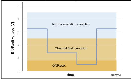
Figure 6. Enable/Fault pin status
