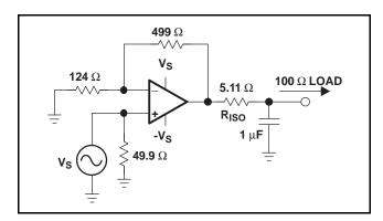
Figure 52. Resistor to Isolate Capacitive Load
