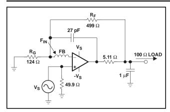
Figure 55. Feedback Technique with Input Ferrite Bead for Capacitive Load
