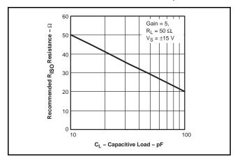
Figure 51. Recommended R<sub>ISO</sub> vs Capacitive Load
