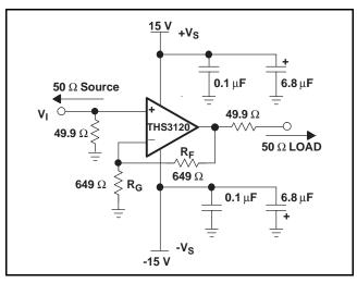
Figure 47. Wideband, Noninverting Gain Configuration
