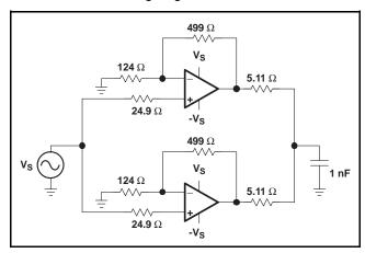
Figure 56. Parallel Amplifiers for Higher Output
