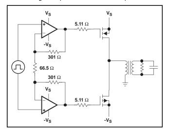
Figure 57. PowerFET Drive Circuit
