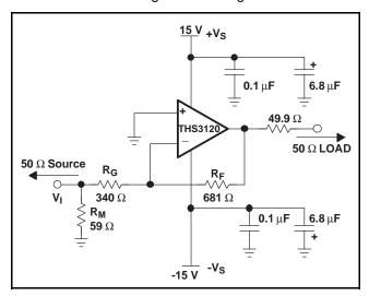
Figure 48. Wideband, Inverting Gain Configuration
