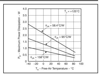
Results are with no air flow and PCB size = 3 inches  $\times$  3 inches (76,2 mm  $\times$  76,2 mm);  $\theta_{JA}$  = 58.4°C/W for MSOP-8 with PowerPAD (DGN);  $\theta_{JA}$  = 95°C/W for SOIC-8 High-K test PCB (D);  $\theta_{JA}$  = 158°C/W for MSOP-8 with PowerPAD without solder.
