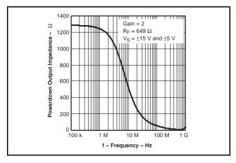
Figure 58. Power-down Output Impedance vs Frequency
