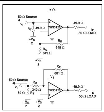
Figure 49. DC-Coupled, Single-Supply Operation
