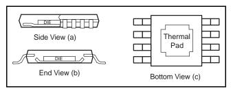
Figure 59. Views of Thermally-Enhanced Package
