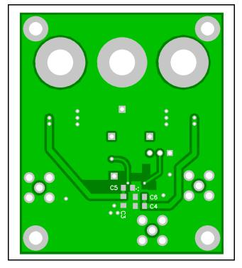
Figure 64. THS3120 EVM Board Layout (Bottom Layer)
