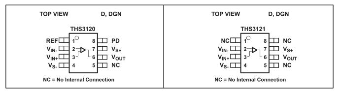
NOTE: The device with the power down option defaults to the ON state if no signal is applied to the PD pin. Additionally, the REF pin functional range is from  $V_{S-}$  to  $(V_{S+} - 4 \text{ V})$ .
