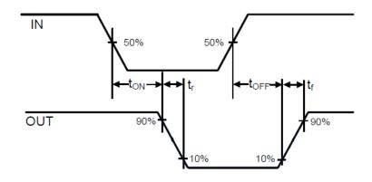
Figure 1. Switching Time Waveform Definitions
