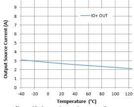
Figure 13. Output Source Current vs. Temperature
