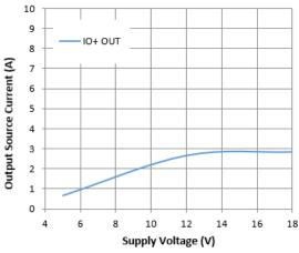
Figure 12. Output Source Current vs. Supply Voltage
