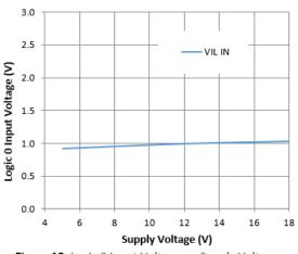
Figure 18. Logic 0 Input Voltage vs. Supply Voltage
