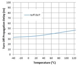
Figure 5. Turn-off Propagation Delay vs. Temperature
