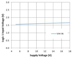
Figure 16. Logic 1 Input Voltage vs. Supply Voltage
