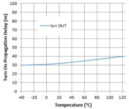
Figure 3. Turn-on Propagation Delay vs. Temperature
