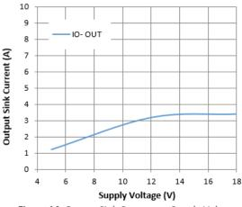
Figure 14. Output Sink Current vs. Supply Voltage
