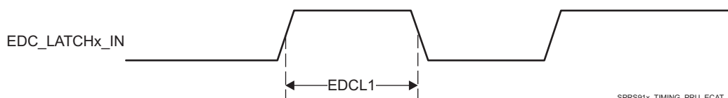
Figure 5-69. PRU-ICSS ECAT LATCHx_IN Timing
