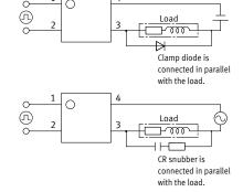
2) When Clamp diode or CR Snubber is used in the circuit, the spike voltages from the load are limited. But the longer wire may become the inductance and cause the spike voltage. Keep the wire as short as possible.
