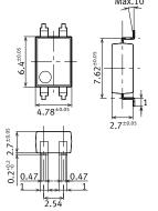
Terminal thickness: t = 0.2General tolerance: ±0.1 PC board pattern (BOTTOM VIEW)
