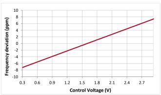
Figure 25. VCTCXO frequency pull characteristic
