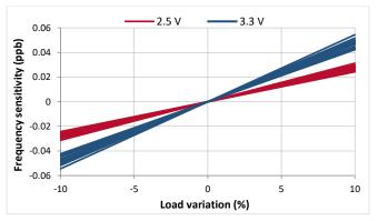
Figure 28. Load sensitivity (±0.1 ppm)
