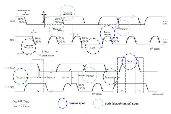
Figure 59. I<sup>2</sup>C Timing Diagram
