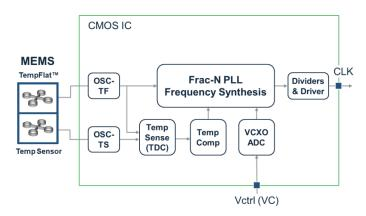
Figure 47. Block Diagram - VCTCXO
