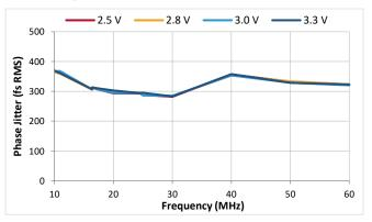
Figure 42. RMS Phase Jitter, DCTCXO, TCXO (Clip Sine)
