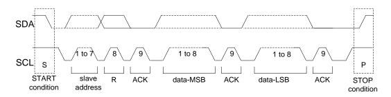
Figure 57. Parallel data byte format, read operation
