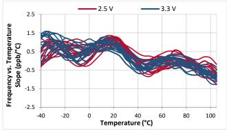
Figure 24. Freq. vs. Temp. Slope (ΔF/ΔT), ±0.1 ppm device
