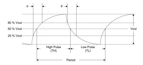
Figure 16. Clipped Sinewave Waveform Diagram<sup>[13]</sup>
