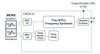
Figure 46. Block Diagram - TCXO
