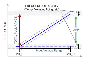
Figure 51. Typical SiTime VCTCXO FV Characteristic
