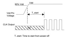
Figure 17. Startup Timing
