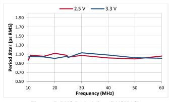
Figure 35. RMS Period Jitter (LVCMOS)
