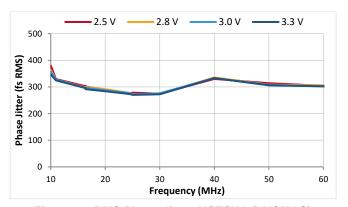
Figure 37. RMS Phase Jitter, VCTCXO (LVCMOS)
