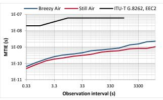
Figure 22. MTIE (0.1 Hz loop bandwidth, ±0.1 ppm) [14]
