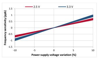
Figure 29. VDD sensitivity (±0.1 ppm)
