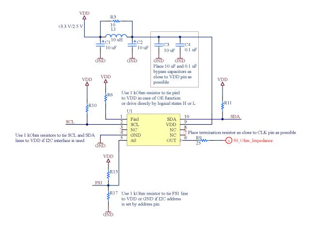
Figure 60. DCTCXO schematic example
