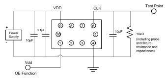
Figure 6. LVCMOS Test Circuit (OE Function)
