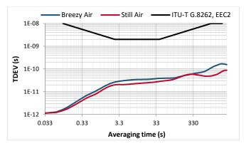
Figure 21. TDEV (0.1 Hz loop bandwidth, ±0.1 ppm) [14]
