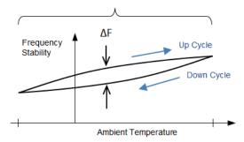
Figure 19. Illustration of hysteresis, where  $\Delta F$  is max frequency difference between up and down cycles across temperature
