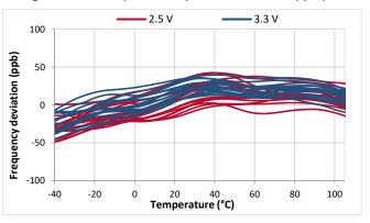
Figure 23. Frequency vs Temperature (±0.1 ppm), 105°C
