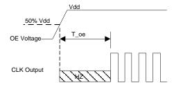
T\_oe: Time to re-enable the clock output
