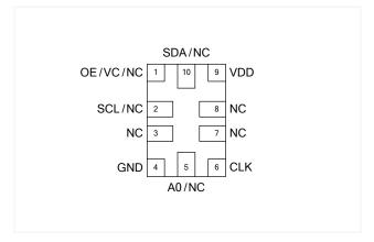
Figure 2. Pin Assignments (Top view)
