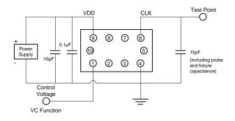
Figure 8. LVCMOS Test Circuit (VC Function)
