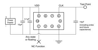
Figure 10. LVCMOS Test Circuit (NC Function)
