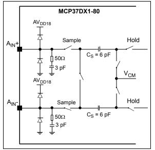
FIGURE 4-2: Equivalent Input Circuit.
