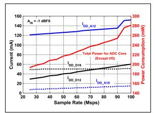
FIGURE 3-47: Power Consumption vs. Sample Rate (LVDS Mode).
