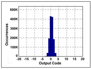
**FIGURE 3-45:** Shorted Input Histogram:  $f_S = 80 \text{ Msps}, \text{MCP37D21-80}.$
