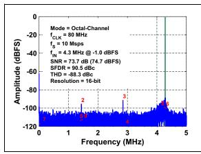
**FIGURE 3-7:** FFT for 4.3 MHz Input Signal:  $f_S = 10$  Msps, Octal-Ch.,  $A_{IN} = -1$  dBFS.
