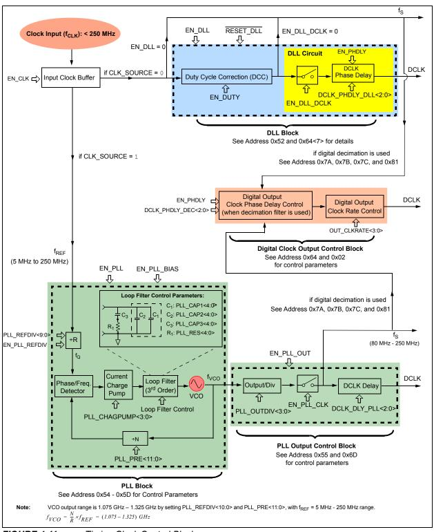
FIGURE 4-11: Timing Clock Control Blocks.
