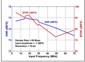
**FIGURE 3-31:** SNR/SFDR vs. Input Frequency:  $f_S = 80$  Msps.
