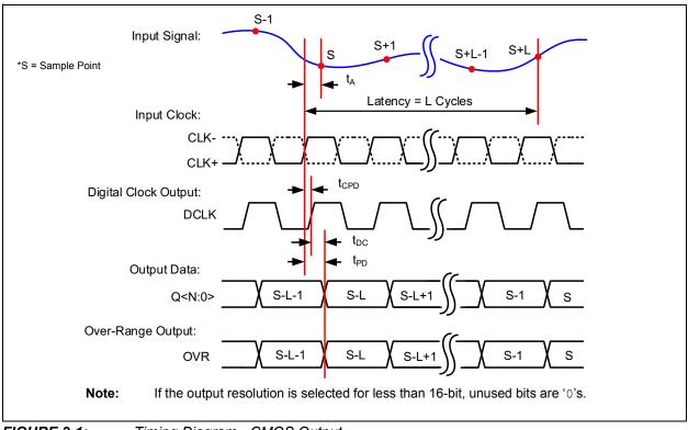
FIGURE 2-1: Timing Diagram - CMOS Output.
