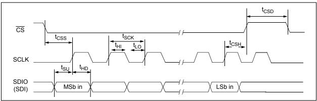
FIGURE 2-5: SPI Serial Input Timing Diagram.
