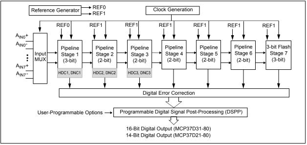
FIGURE 4-1: ADC Core Block Diagram.
