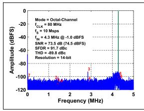
**FIGURE 3-19:** FFT for 4.3 MHz Input Signal:  $f_S = 10$  Msps, Octal-Ch.,  $A_{IN} = -1$  dBFS.
