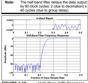
FIGURE 4-19: High-Pass (HP) Response of Half-Band Filter.
