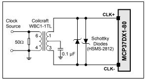
**FIGURE 4-9:** Transformer-Coupled Differential Clock Input Configuration.
