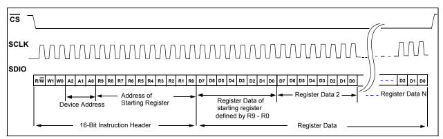
**FIGURE 5-1:** SPI Serial Data Communication Protocol with MSb-first. See Figures 2-5 and 2-6 for Timing Specifications.
