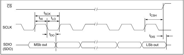
FIGURE 2-6: SPI Serial Output Timing Diagram.
