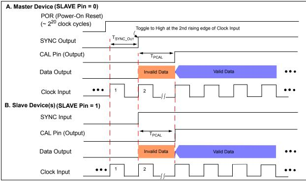
FIGURE 2-9: Sync Timing Diagram with Power-On Reset.
