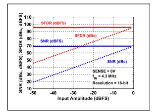
**FIGURE 3-28:** SNR/SFDR vs. Analog Input Amplitude:  $f_S = 80$  Msps,  $f_{IN} = 4.3$  MHz, Low-Reference Mode (SENSE = GND).
