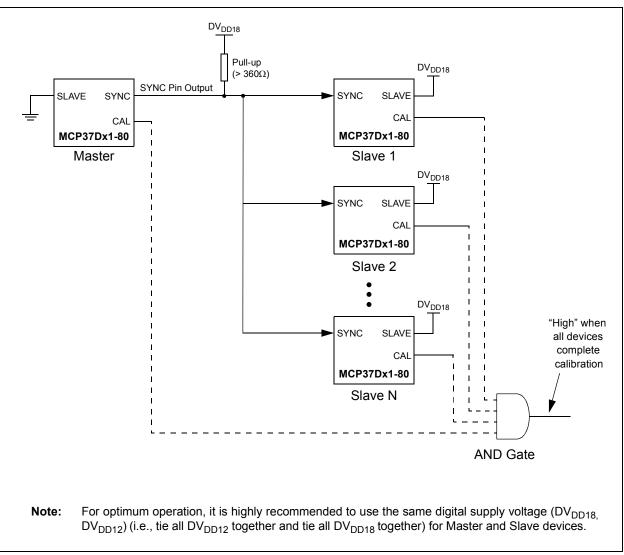
FIGURE 4-27: Synchronizing Multiple ADCs Using AutoSync Feature.
