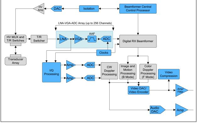
FIGURE 4-22: Example of Ultrasound System Building Block.
