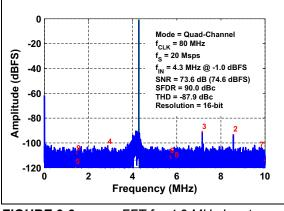
**FIGURE 3-3:** FFT for 4.3 MHz Input Signal:  $f_S = 20$  Msps, Quad-Ch.,  $A_{IN} = -1$  dBFS.
