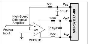
**FIGURE 4-4:** DC-Coupled Input Configuration with Preamplifier: the external signal conditioning circuit and associated component values are for reference only. Typically, the amplifier manufacturer provides reference circuits and component values.
