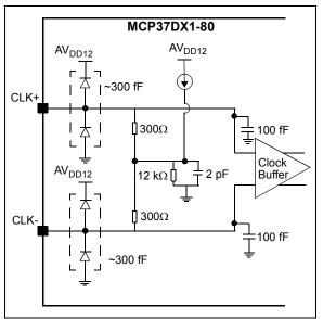
FIGURE 4-8: Equivalent Clock Input Circuit.
