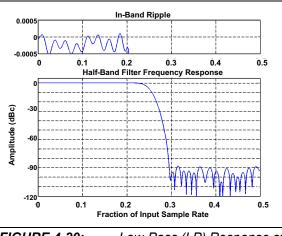
FIGURE 4-20: Low-Pass (LP) Response of Half-Band Filter.
