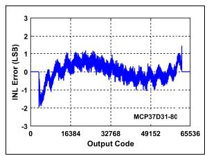
**FIGURE 3-40:** INL Error Vs. Output Code:  $f_S = 80 \text{ Msps}, f_{IN} = 4.3 \text{ MHz}, A_{IN} = -1dBFS,$ MCP37D31-80.
