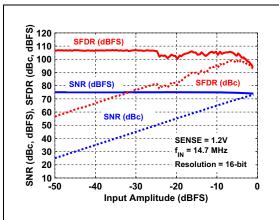
FIGURE 3-25:SNR/SFDR vs. Analog InputAmplitude:  $f_S = 80$  Msps,  $f_{IN} = 14.7$  MHz,High-Reference Mode (SENSE =  $AV_{DD12}$ ).
