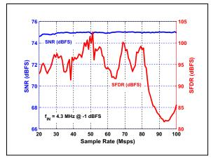
**FIGURE 3-30:** SNR/SFDR vs. Sample Rate (Msps):  $f_{IN} = 4.3$  MHz.
