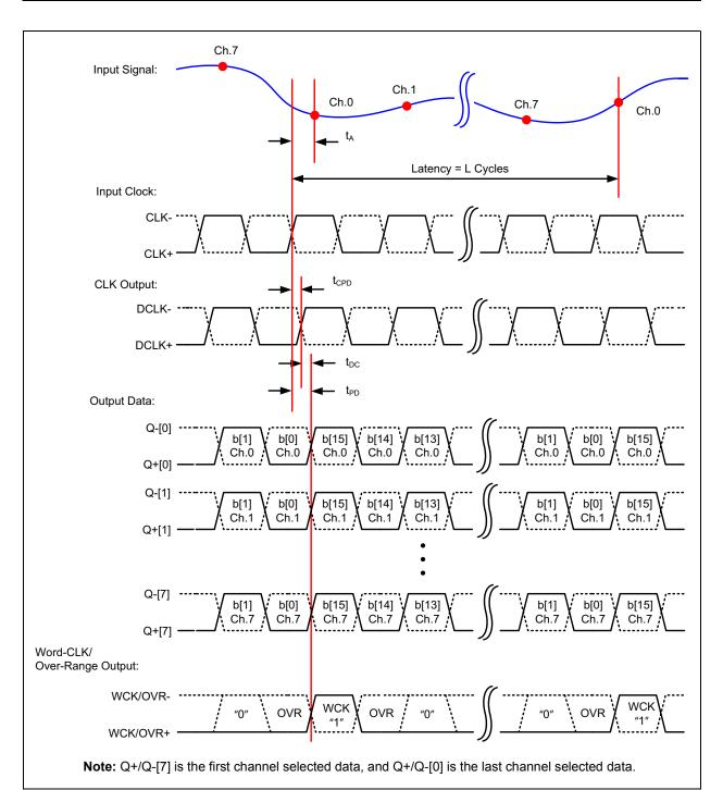
**FIGURE 2-4:** Timing Diagram - LVDS Serial Output in Octal-Channel Mode. This output is available for octal-channel with 16-bit mode only. Note that although the eight input channels are sampled sequentially (auto-scan with 1 cycle separation), all channels are output simultaneously with the MSb (bit 15) synchronized with the rising edge of WCK.
