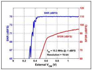
**FIGURE 3-34:** SNR/SFDR vs.  $V_{CM}$  Voltage (Externally Applied):  $f_S = 80$  Msps,  $f_{IN} = 15.3$  MHz.
