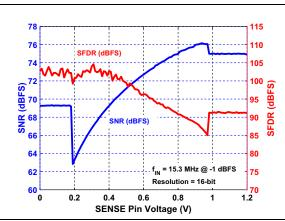
**FIGURE 3-32:** SNR/SFDR vs. SENSE Pin Voltage:  $f_{IN}$  = 15.3 MHz.
