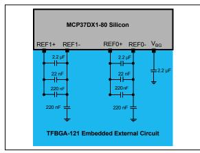
FIGURE 4-7:Embedded DecouplingCircuit in TFBGA-121 Package for VoltageReference and  $V_{BG}$  pins. No external circuit isrequired on an application PCB.
