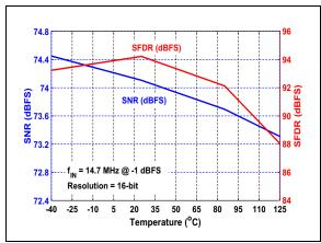
**FIGURE 3-35:** SNR/SFDR vs. Temperature:  $f_S = 80 \text{ Msps}, f_{IN} = 14.7 \text{ MHz}, V_{SENSE} = AV_{DD12}, A_{IN} = -1 \text{ dBFS}.$
